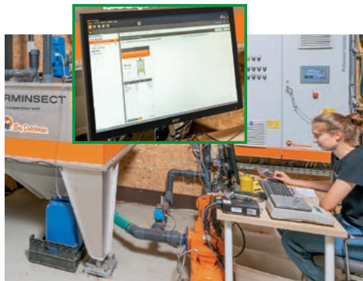
The feed mash is mixed in two mixing tanks, controlled by a computer. Both mixing tanks are placed on load cells for this purpose
