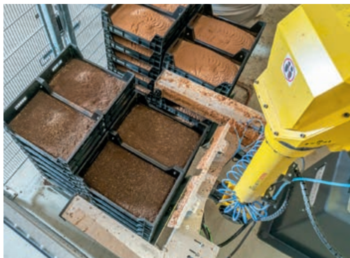
... takes two crates with fully-grown larvae from the pallet on the other side ...
