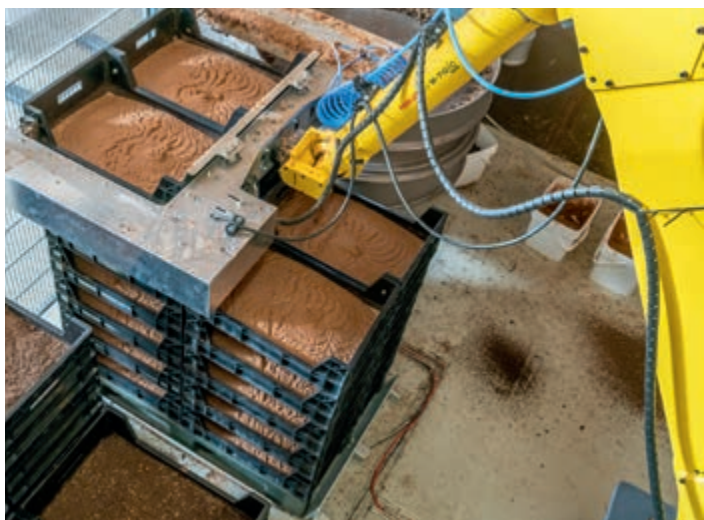
The robot stacks the crates with the feed mash on a pallet, ...
