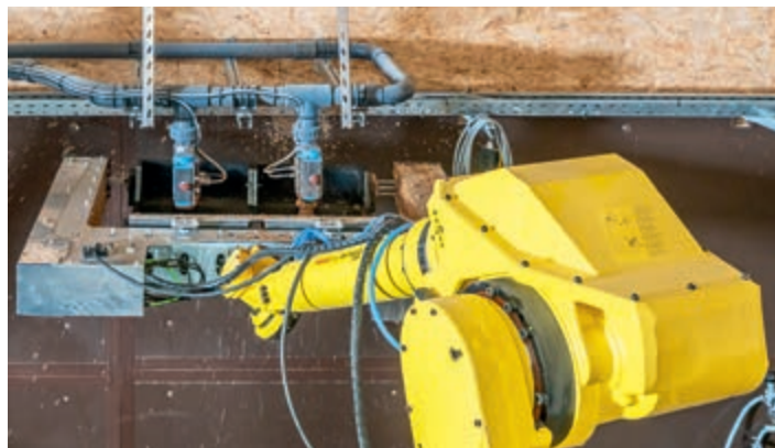
Two feed valves dispense the fresh feed required for one week of larvae growth
